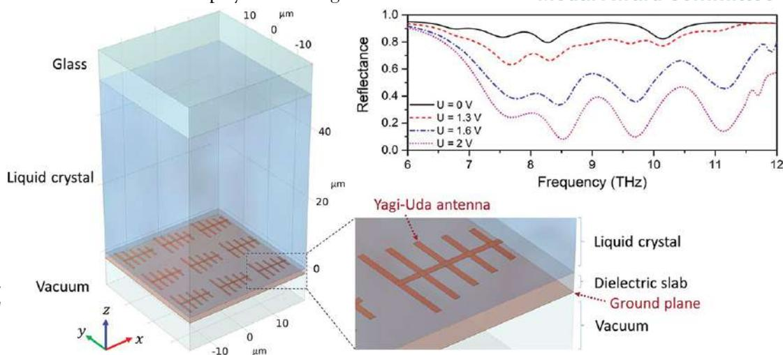
Tuning Yagi-Uda antennas array reflectance with help of liquid crystal from [17].
